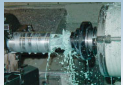
Cutting multiple keyways on a machining center.
