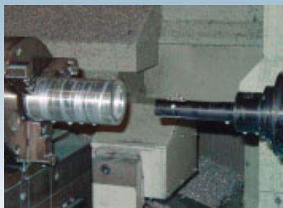
Cutting multiple keyways on a machining center.
